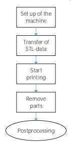
Setup machine for the resin (Settings see machine manual) and fill the polymer tray/basement. To avoid impurities, resin mixes and contamination a separate polymer tray/basement must be used \*.
